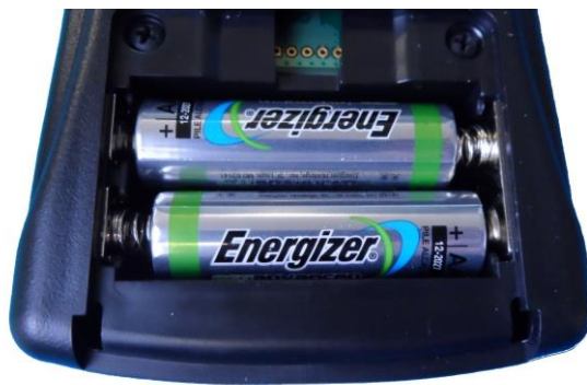
Figure 7: Two AA batteries correctly fitted
