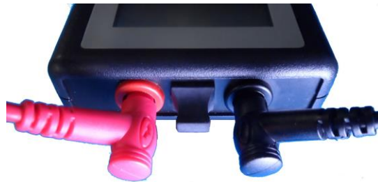
Figure 11: Test leads connected ready to read copper IRIG-B signals
